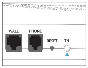
1) Press the white T/L button on the rear of the Base Unit.
