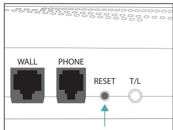
4) On the rear of the Base Unit, press the black RESET button once. Now test your Wall Button by pressing it once. Please wait for the unit to connect to the monitoring center. Advise the dispatcher that you are testing.
