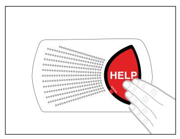
2) Then press the large, red HELP button on the Base Unit twice. Make sure you hear it say "Group 2." If you don't hear it, press the RESET button and start from Step 1.
