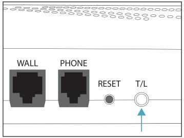
On the rear of the Base Unit, press the T/L button one time. The unit will announce, "Range Test Mode."
