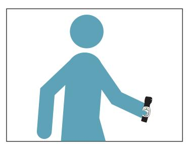
3) For Personal Help Buttons, walk around all areas of the home and yard while holding it down. Listen for the steady tone from the Base Unit. For Wall Buttons, hold the button down in the area where you want to place the button. Take note of any areas where the tone stops. The stops indicate that the button cannot call for help in that area.
