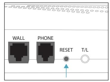
4) Once all areas are tested, stop pressing down the button. Then press the black "RESET" button on the rear of the Base Unit. It will announce, "System Ready." If stops were detected, try relocating the Base Unit and perform the test again, and/or contact your service provider.
