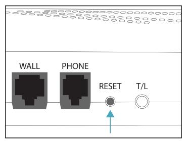
4) On the rear of the Base Unit, press the black RESET button once. Now test your Personal Help Button once. Please wait for the unit to connect to the monitoring center. Advise the dispatcher that you are testing.
