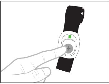
2) Immediately press and hold down the button. A steady tone will sound from the Base Unit. This means the unit is detecting the button.
