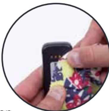
Take a soft cloth, such as an eyeglass cleaning cloth, and gently rub the gold contacts on the device and charging cradle to remove dirt, oil and debris.
