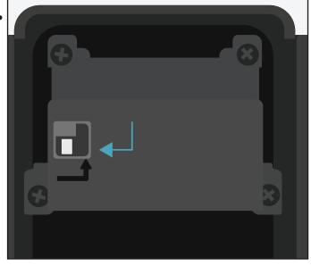
Move the silver lever back down to its default position. Be sure not to rotate the combination when moving the lever back.
