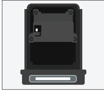
Turn over the Lockbox and pull back the silver loop to open the Lockbox.
